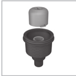
– Vertical drain connection fitting with removable siphon trap, sealing water height 50 mm, DN 50
